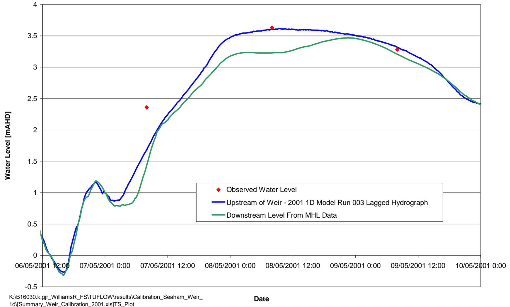
Figure 6-5 Seaham Weir Loss Calibration – May 2001
