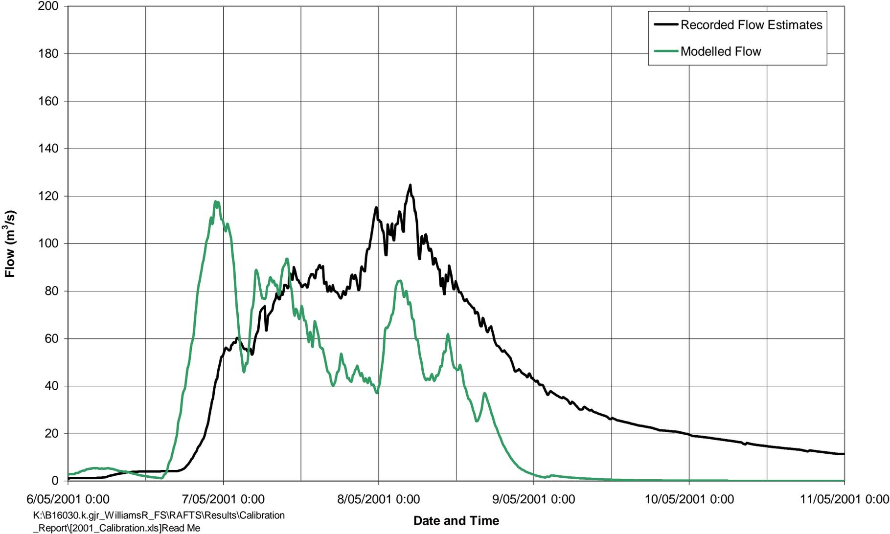
Figure 5-13 May 2001: Wangat Gauge Comparison for Hydrological Model
