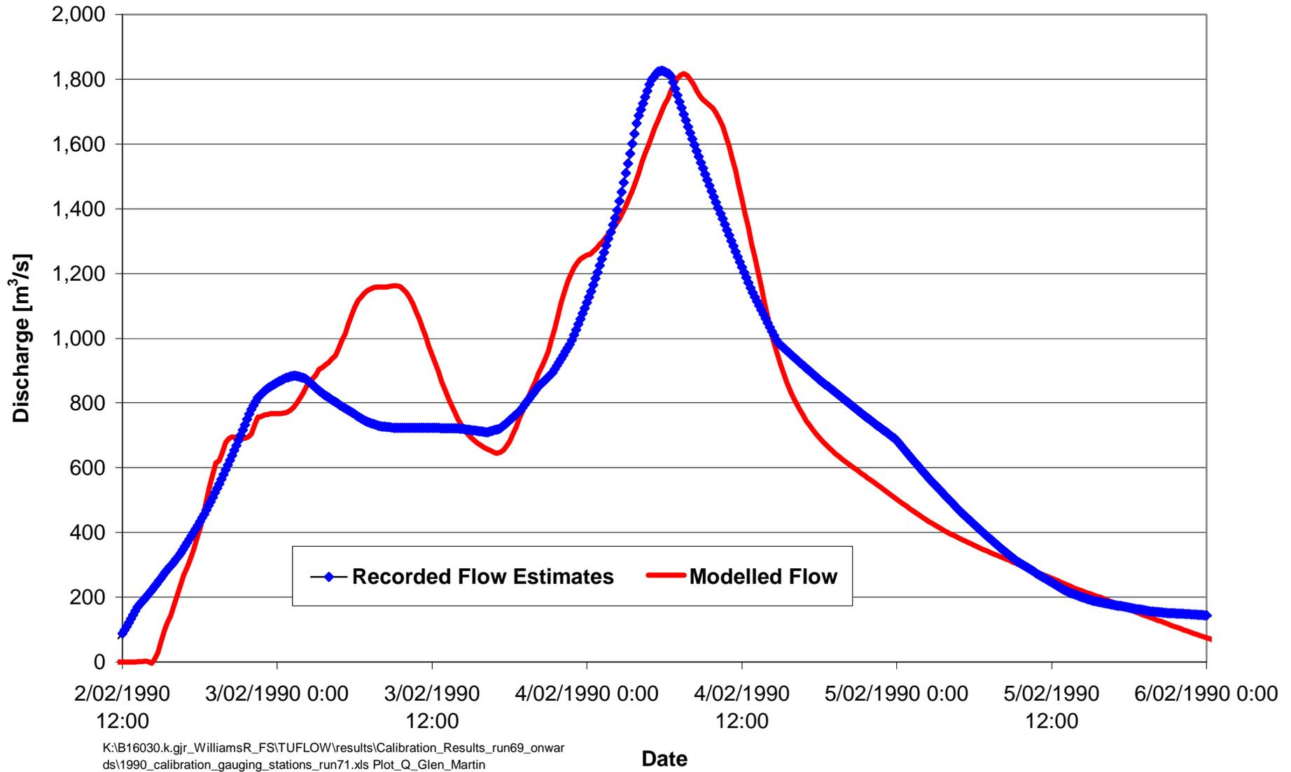
Figure 6-16 February 1990: Glen Martin Gauge Flows Comparison for Hydraulic Model
