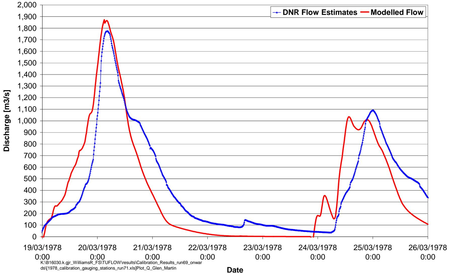
Figure 6-10 March 1978: Glen Martin Gauge Flows Comparison for Hydraulic Model
