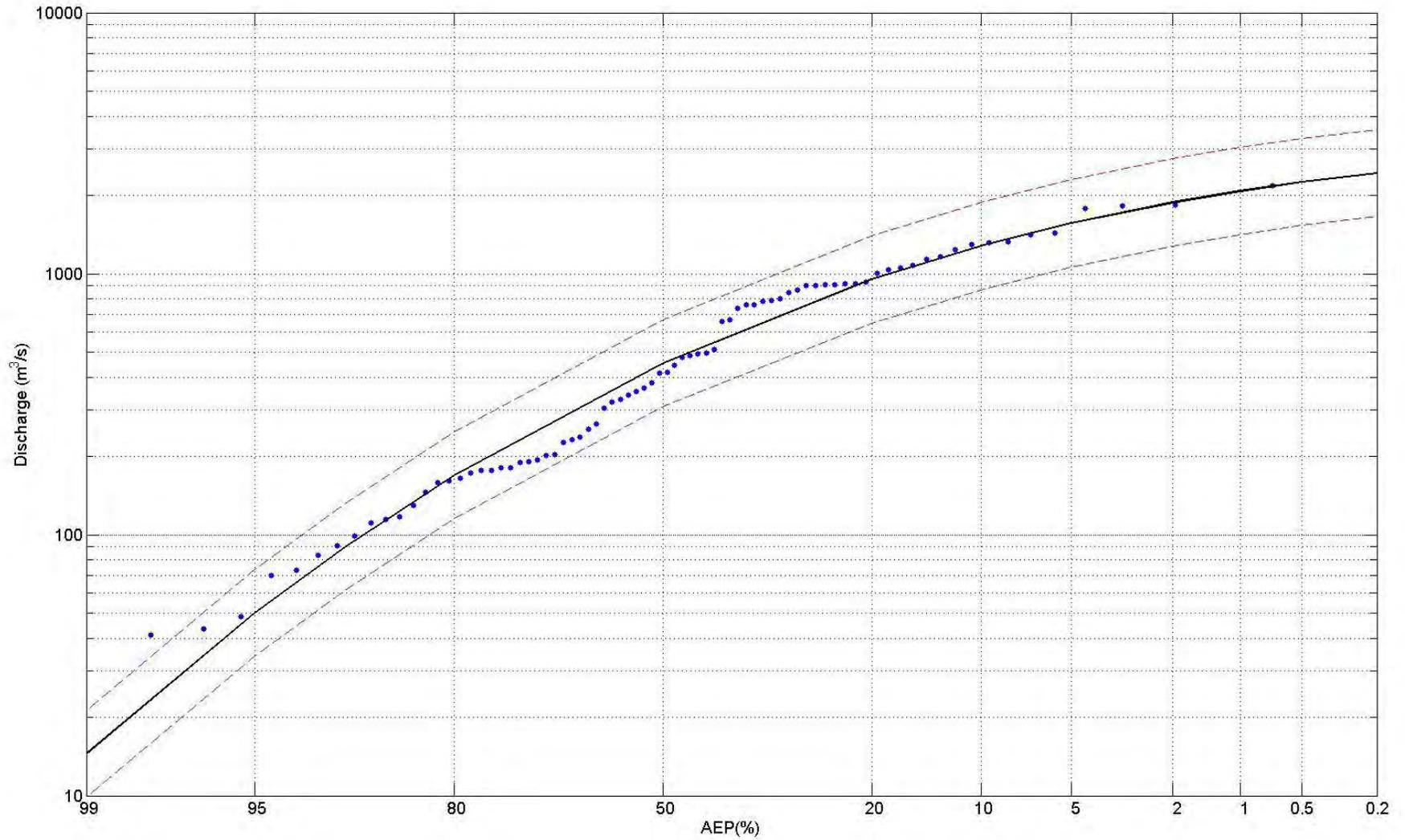
Figure 5-20 LPIII Distribution Fitted to Glen Martin Annual Maximum Discharge Series
