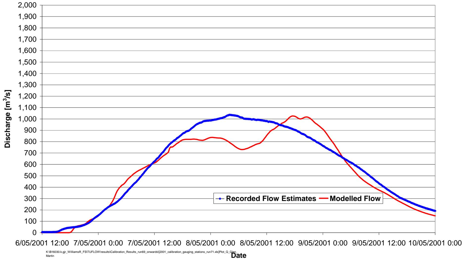
Figure 6-26 May 2001: Glen Martin Gauge Flows Comparison for Hydraulic Model
