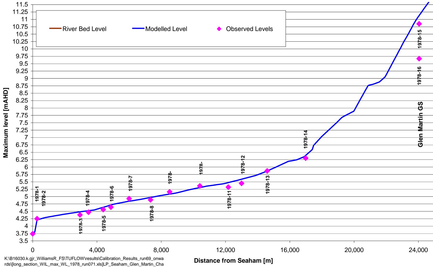
Figure 6-12 March 1978: Long Section Comparison for Hydraulic Model – Seaham to Glen Martin
