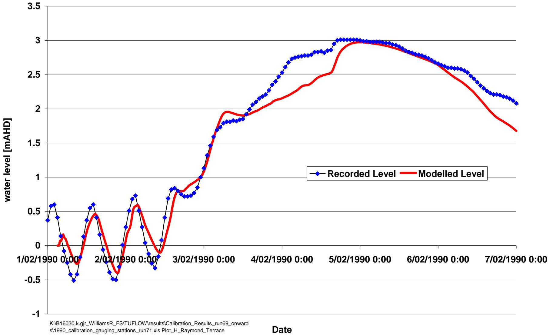
Figure 6-18 February 1990: Raymond Terrace Gauge Levels Comparison for Hydraulic Model
