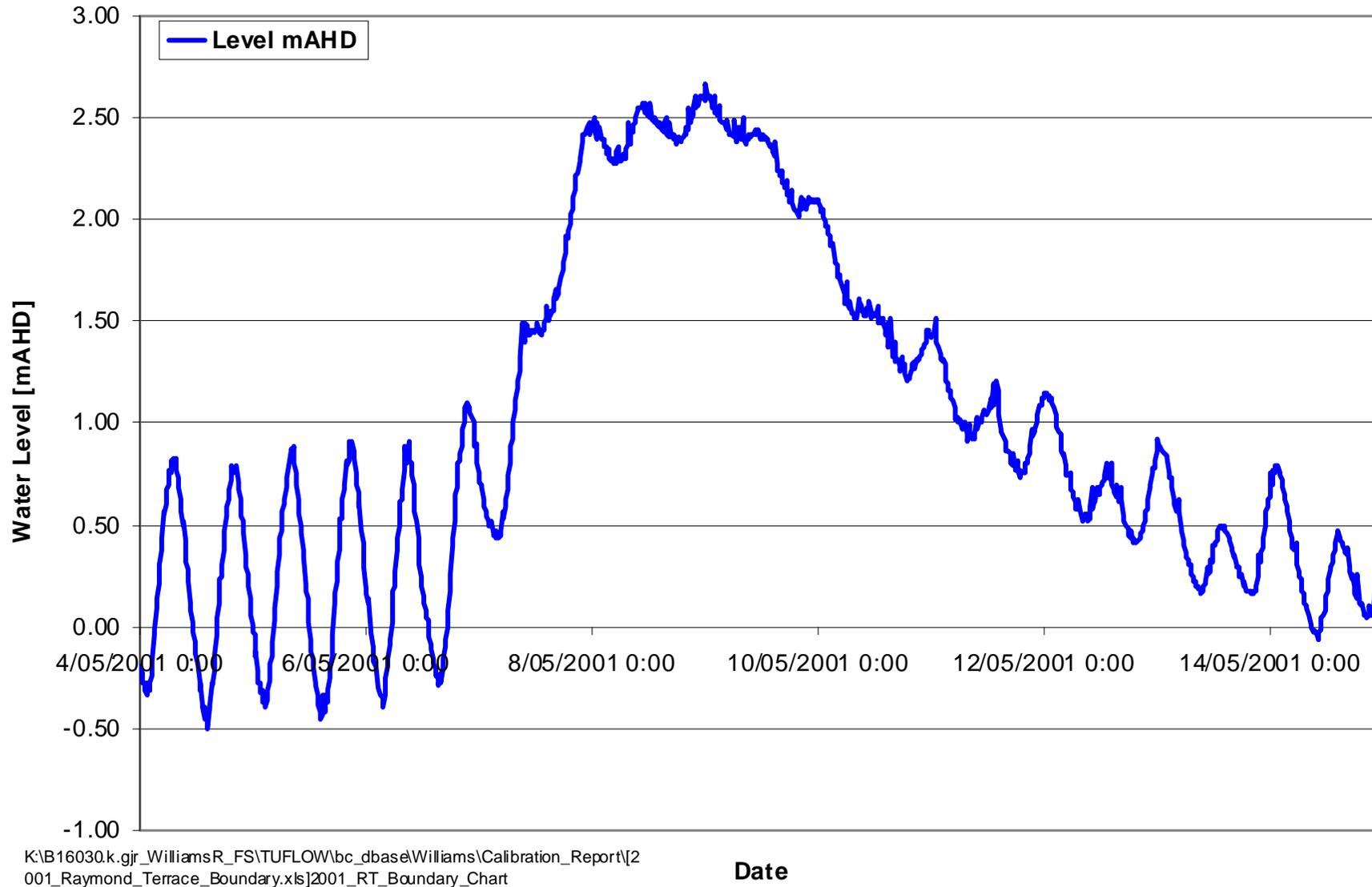
Figure 6-23 Raymond Terrace Recorded Levels as Boundary Condition for May 2001 Flood
