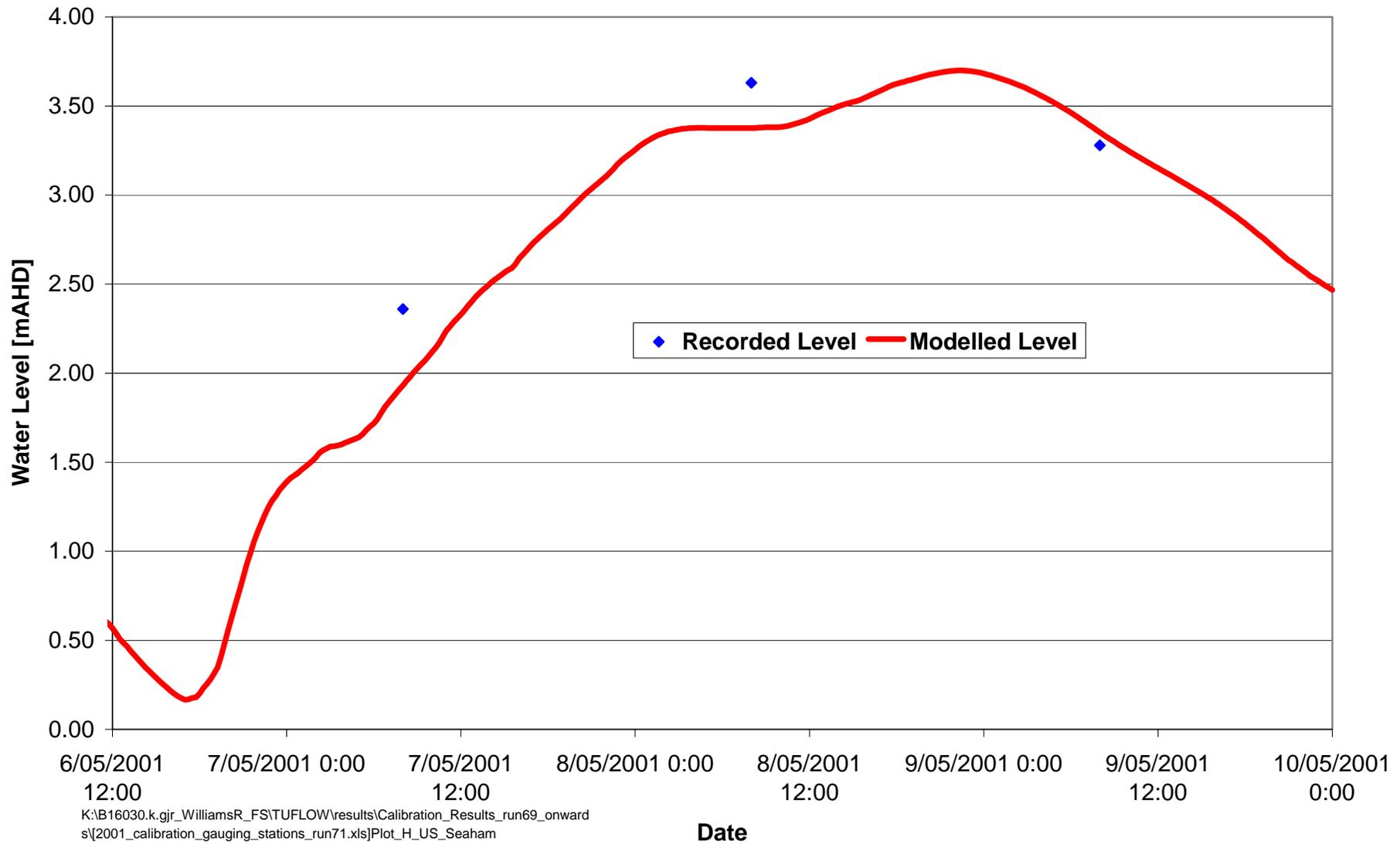
Figure 6-27 May 2001: Upstream Seaham Weir Levels Comparison for Hydraulic Model
