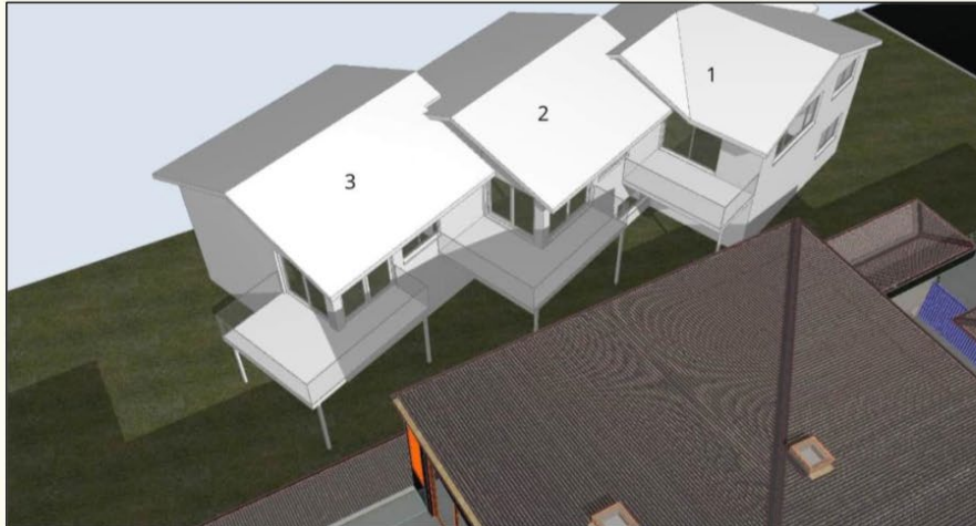
Figure 13. Elevation shadows for 11am showing direct sunlight to at least 50% of Unit 3 POS and almost 50% of Unit 1 POS
