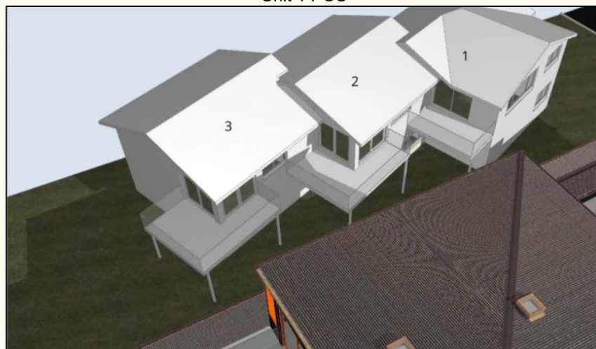
Figure 15. Elevation shadows from 1pm showing direct sunlight to at least 50% of Unit 1 POS
