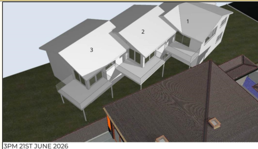
Figure 17. Elevation shadows from 3pm showing direct sunlight to at least 50% of Unit 1 and 2 POS
