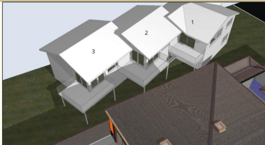
Figure 15. Elevation shadows from 1pm showing direct sunlight to at least 50% of Unit 1 POS
