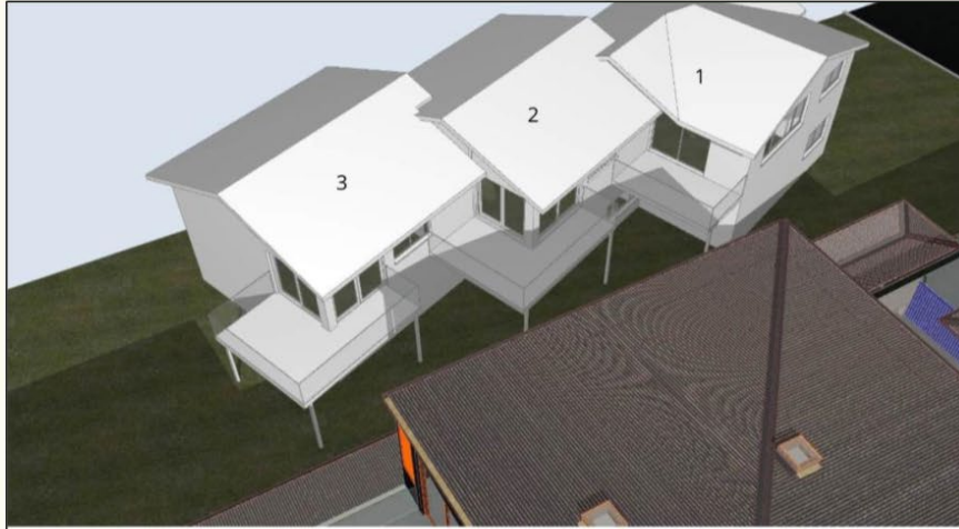
Figure 13. Elevation shadows for 11am showing direct sunlight to at least 50% of Unit 3 POS and almost 50% of Unit 1 POS
