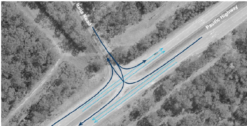
Figure 4: Existing Intersection Layout (Source: Applicants documentation)
