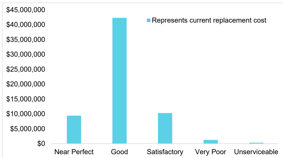
Figure 9: Condition Rating – Kerbs and Guttering
