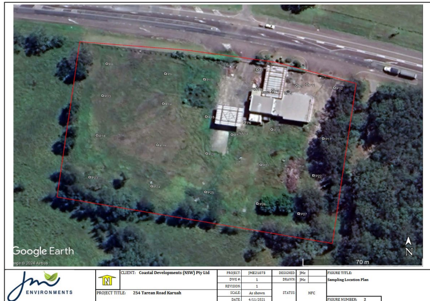
Figure 3: Borehole testing locations (source: JM Environments, 2024)
