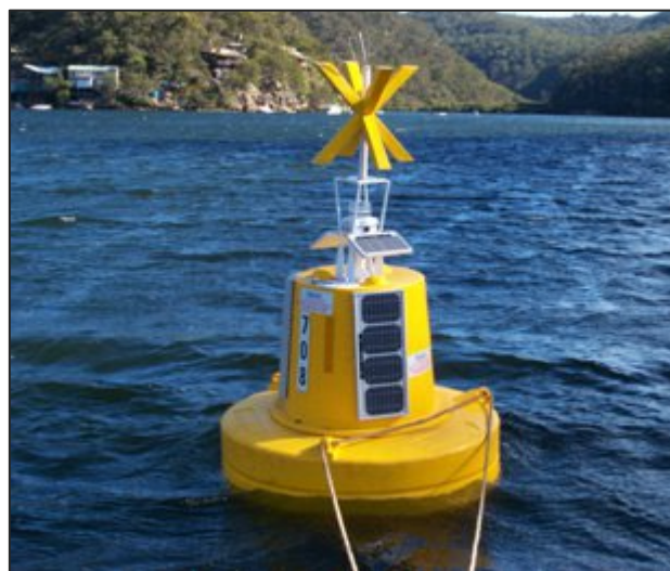
Image: water quality buoy (source: https://mhl.nsw.gov.au/DataCollection )
