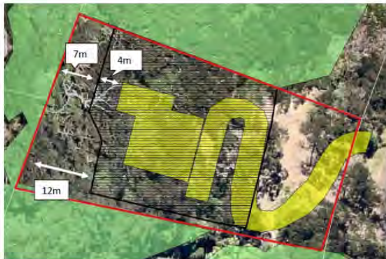
Figure 6: Plan of the site, showing the area of bushfire threat in green and the proposed dwelling and driveway in yellow, with the proposed APZ being identified by the black hatched area
