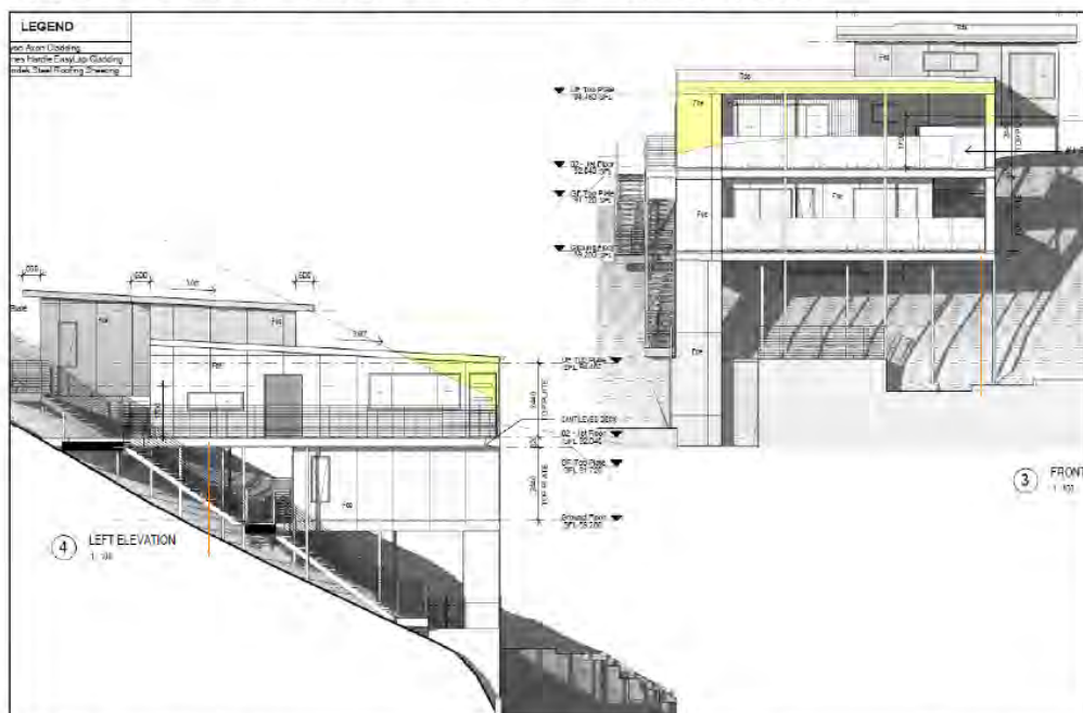
Figure 1: Elevation plan of the proposed dwelling, with the yellow area indicating the area above the 9m height limit
