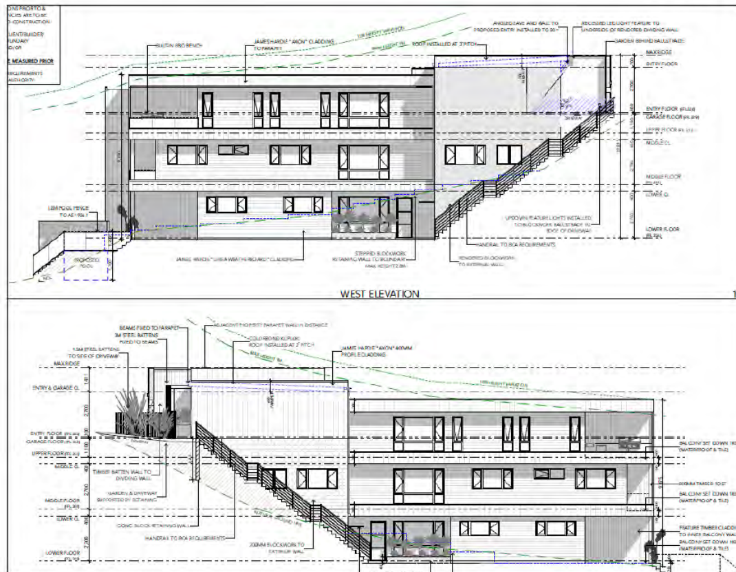
Figure 1: Elevation plans showing the dwellings and the proposed height exceedance, with the natural ground level and corresponding height limit shown by a green dashed line and the proposed retaining walls shown by the blue dashed line
