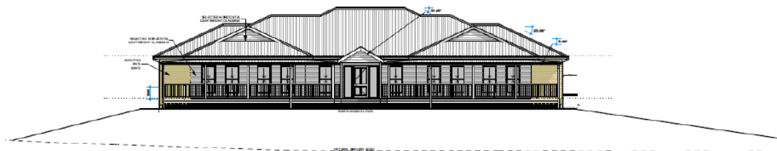
Figure 1: North-west elevation of proposed dwelling
