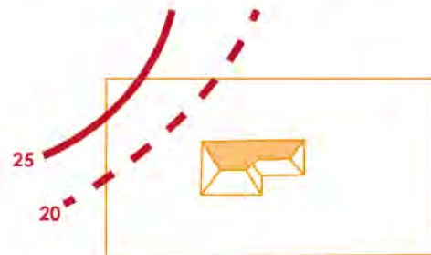
Figure BL: Illustration of Building Site Acceptability based on ANEF Zone
