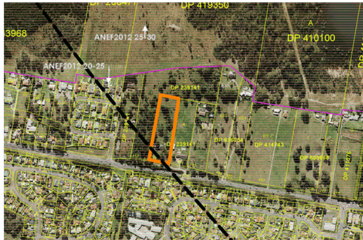
Figure 10: Illustrating the boundary between 'Conditionally Acceptable' and 'Unacceptable' in accordance with ANEF 2012.
