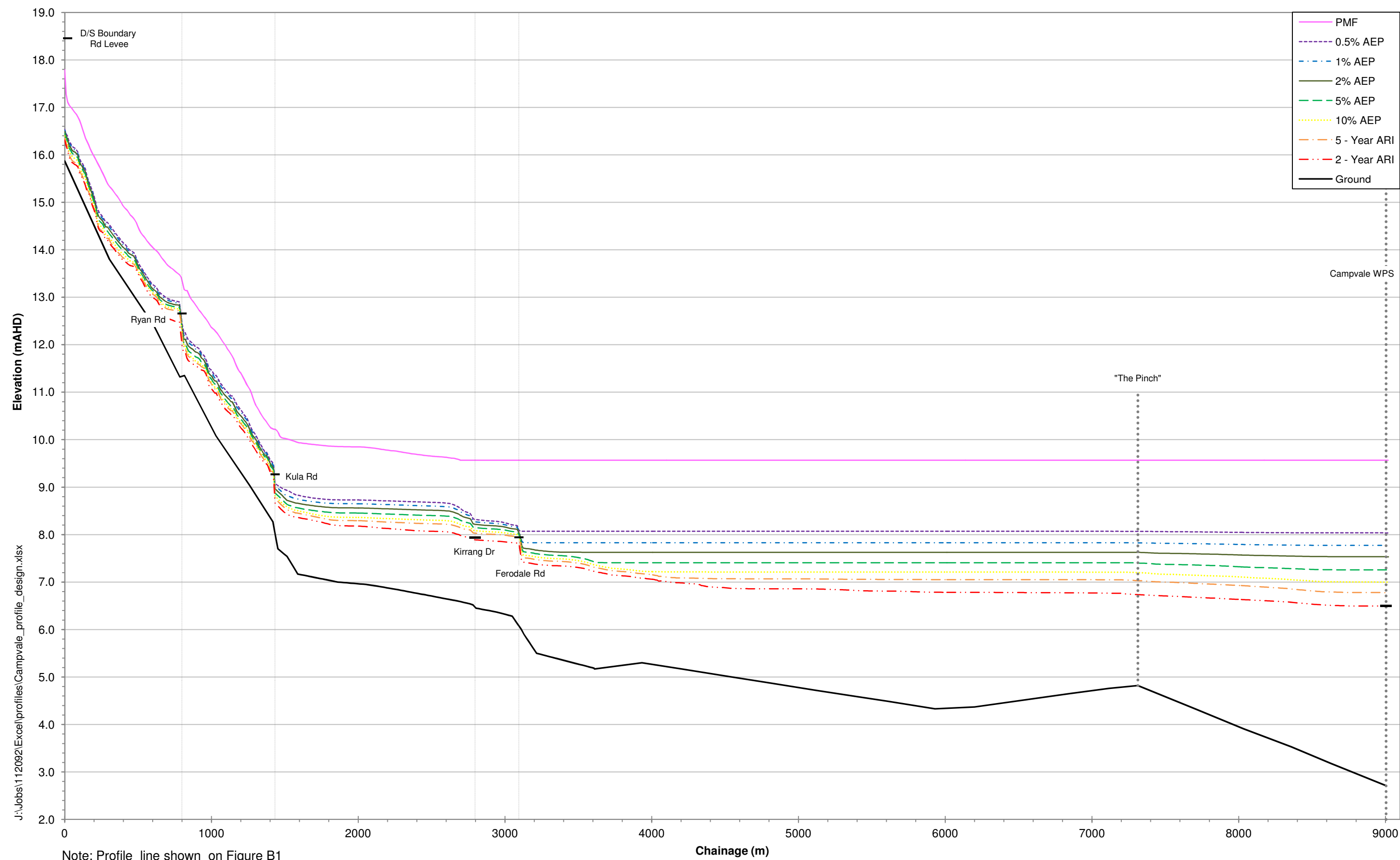
FIGURE C9 CAMPVALE DRAIN - DESIGN FLOOD PROFILES
