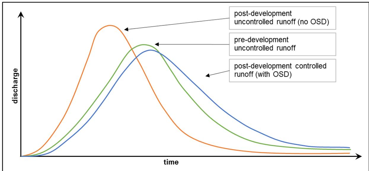
Runoff does not necessarily need to be attenuated in a basin. On a small scale, storage areas can include flooding above ground to shallow depths such as in parking areas or garden features. Storage can also be provided in underground systems which can reduce above ground nuisance flooding to land owners. On a larger scale, basins are often used for communal provision of OSD.
